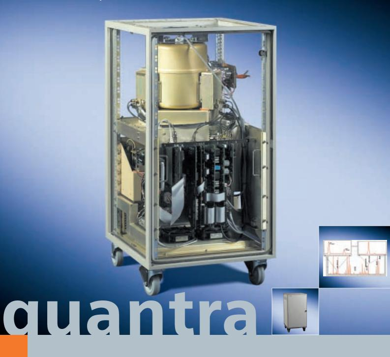
Ion Cyclotron Resonance Mass Spectrometry provides unparalleled mass resolution. With a mass resolution of 20,000, which is orders of magnitude better than for typical mass spectrometers, the QUANTRA can identify compounds with nearly identical masses. Applications that used to require laborious front-end preparations are now possible with ICR Mass Spectrometry.
